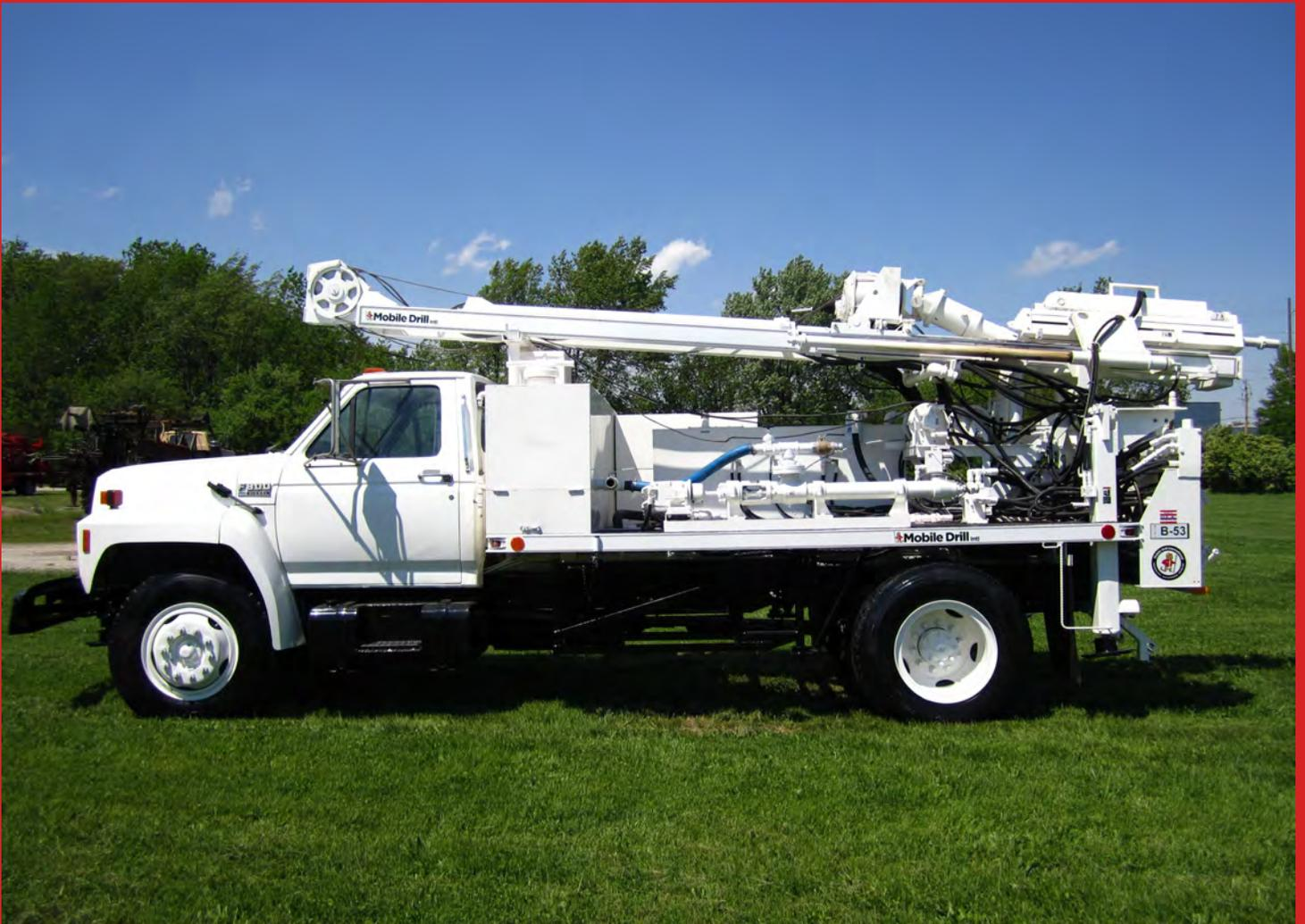
The B53 is a compact, hydraulic drill with applications in geotechnical, environmental and mineral exploration. Auger drilling, both hollow stem and continuous flight, rotary and diamond core drilling and angle drilling are all possible. The B53 is sized for mounting on a variety of carriers to provide go-anywhere versatility. The B53 can be powered either from a carrier engine PTO or a dedicated drill engine.
